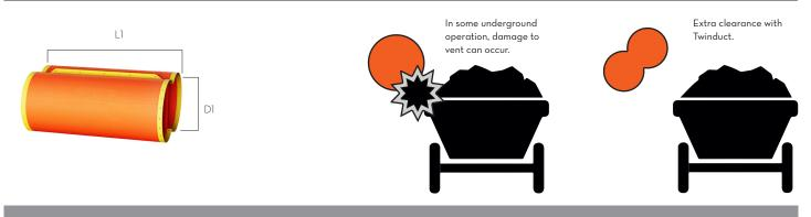
Twinduct is designed to be used in areas where damage is likely to occur on tight areas of underground mining, especially where mine tunnel heights are limited.
