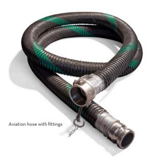
Note: This hose is not recommended for use close to direct external radiant heat as the cover is not flame-retardant. Hoses should be flushed with diesel or kerosene after use. Cleaning with steam or direct external heat is not recommended.
